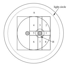
Fig. 1. The 2d HRWE problem and its domain decomposition. The circles that are the outer boundaries of the darkened source regions carry Dirichlet boundary conditions representing the imprint of the sources. Region H, between the two small circles concentric with the source, is the inner annular domain. Domain A between two large solid circles is the outer annular domain. The dashed circle in domain A is the light circle.
